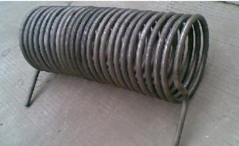
The heat-exchanger coil made of ASTM A213 T9 tubes.
